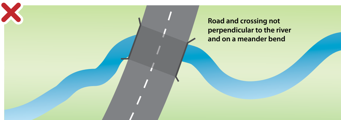
Figure 27: Poor practice, crossing not perpendicular to river and on a meander bend.
